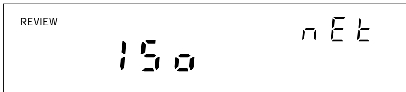
Network display for reviewing the network type (isolated network)
